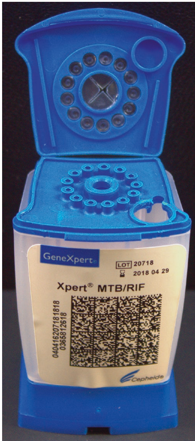
■ Fig. 42.24 Cepheid GeneXpert® MTB/RIF real-time PCR assay cartridge
