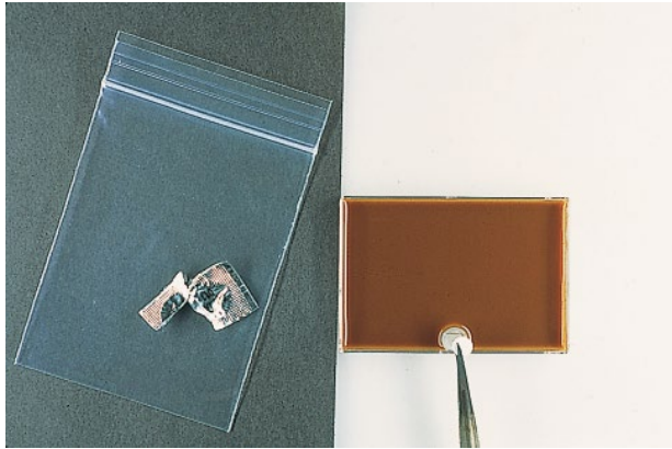
Figure 21-9 JEMBEC plates. The JEMBEC plate shown here contains a selective agar, GC-Lect agar (Thermo Fisher Scientific, Waltham, MA), designed for the enhanced recovery of N. gonorrhoeae . Upon inoculation of the medium with the specimen, a CO 2 -generating tablet consisting of citric acid and sodium bicarbonate is placed in the JEMBEC plate, as shown. The plate is covered, sealed in the plastic bag provided, and transported to the laboratory.
