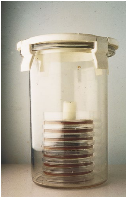
Figure 21-7 Candle jar. Agar plates are placed in a jar, a candle is lit, and the jar is sealed. When the O 2 has been consumed, the candle is extinguished, leaving an atmosphere of 3% CO 2 . Inoculated agar is then transported and incubated at 35 to 37°C in this CO 2 environment. Candle jars are an alternative to commercially available systems for the transport and recovery of N. gonorrhoeae .
