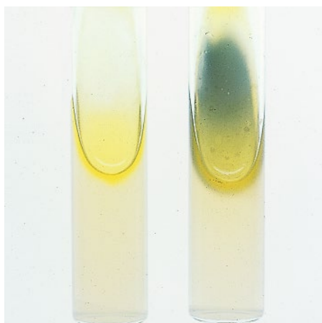
Figure 41-55 Phenylalanine deaminase test. Amino acids can be oxidatively deaminated to form a keto acid. In the presence of phenylalanine deaminase (PAD), the amino acid L-phenylalanine is converted to phenylpyruvic acid, a keto acid. If the slant remains colorless upon the addition of 10% ferric chloride, the test is negative (left). However, if the slant turns green, the test is positive (right). Proteus spp., Providencia spp., and Morganella spp. are PAD positive.
