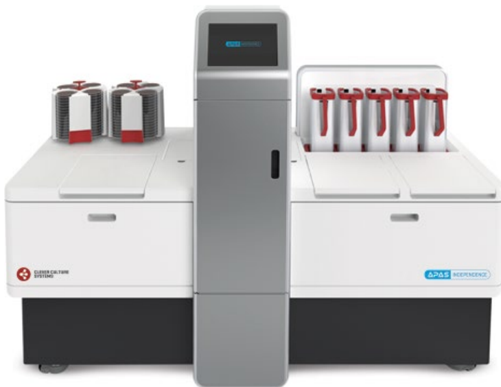
Figure 40-9 APAS Independence. The APAS Independence is a stand-alone system that uses artificial intelligence to automate culture plate imaging, analysis, and interpretation. Space requirements: depth, 2,000 mm; width, 800 mm; height, 1,600 mm; weight, 330 kg. (Photo courtesy of Clever Culture Systems, Zurich, Switzerland.)
