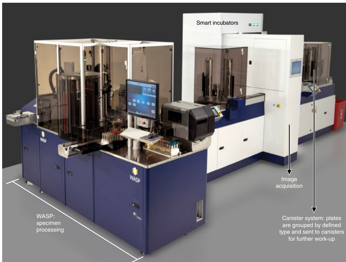
Figure 40-6 WASPLab automated system. The WASPLab system includes different modules connected by a unidirectional conveyor track. The WASP DT includes smart incubation (CO 2 and aerobic), digital microbiology, and artificial intelligence. Single and double smart incubators have the capacity for 795 and 1,590 plates, respectively. The reading of the digital images and additional workup are done on remote workbenches. Space requirements for WASP DT with a single incubator: depth, 1,158 mm; width, 853 mm; height, 2,316 mm; weight, 553 kg. (Photo courtesy of Copan Diagnostics, Murrieta, CA.)
