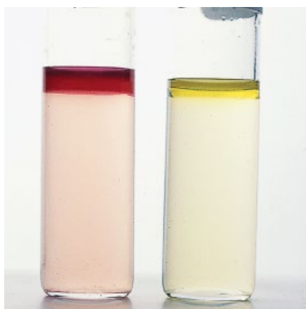
Figure 41-48 Indole test. Some organisms possess the enzyme tryptophanase, which converts tryptophan to indole. Indole is detected by the addition of p -dimethylaminobenzaldehyde (Ehrlich's or Kovac's reagent) to a broth solution (tube test). (A) If a ring of red appears at the interface between the top of the broth and the reagent, the test is positive (left); a negative test is shown on the right. (B) Alternatively, when filter paper impregnated with p -dimethylcinnamaldehyde is used, a negative reaction (left) is colorless, whereas the formation of a green color indicates a positive test (right).
