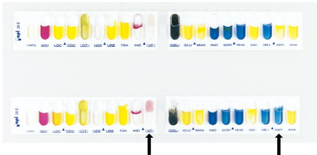
Figure 15-6 Aeromonas hydrophila and Aeromonas caviae identified by the API 20E system. Both A. hydrophila and A. caviae are included in the API 20E (bioMérieux, Inc., Durham, NC) database; therefore, this system can be used to identify these two Aeromonas spp. In this example, A. caviae appears in the top strip and A. hydrophila is in the bottom strip. The reactions that differentiate them, indicated by arrows, are Voges-Proskauer (VP) and amygdalin (AMY). A. hydrophila is VP positive (red), while A. caviae is negative (no color). A. caviae is AMY positive (yellow), while A. hydrophila is negative (blue). The combination of the reactions in each of the strips, as well as the positive oxidase reactions, confirms the identification of these two isolates.
